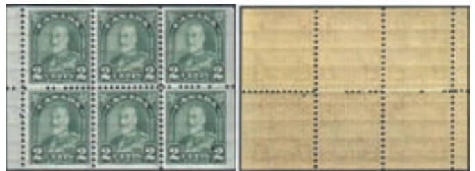
Stickney rotary press wet printed booklet stamps with gum breakers on the rough gum side.
